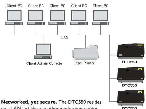
**Networked, yet secure.** The DTC550 resides on a LAN just like any other workgroup printer.
